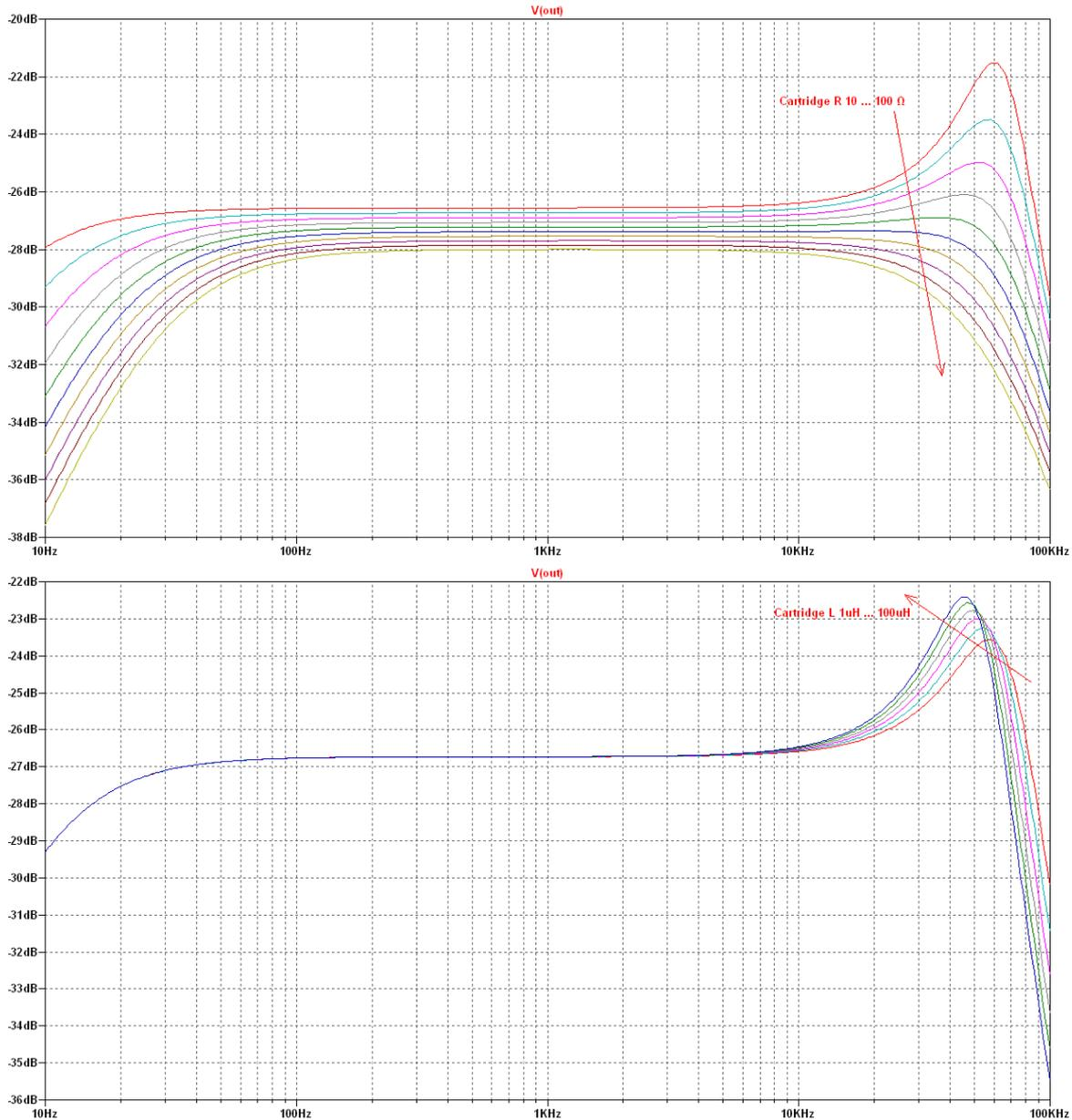
Fig. 3 and 4 Effect of cartridge parameters on the frequency response of the combined system. In figure 3, the low frequency response is impaired for higher  $R_{cartridge}$  that would require higher  $L_p$  for a proper match.
