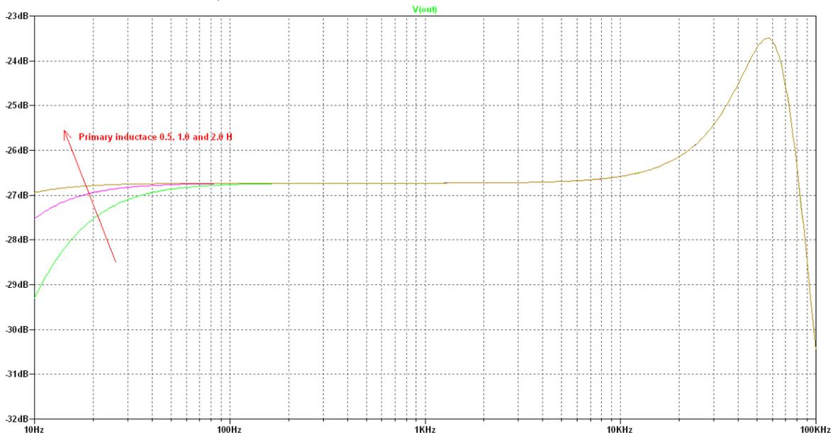
Fig. 8 Higher  $L_p$  extends into deeper bass the transformer's bandwidth.
