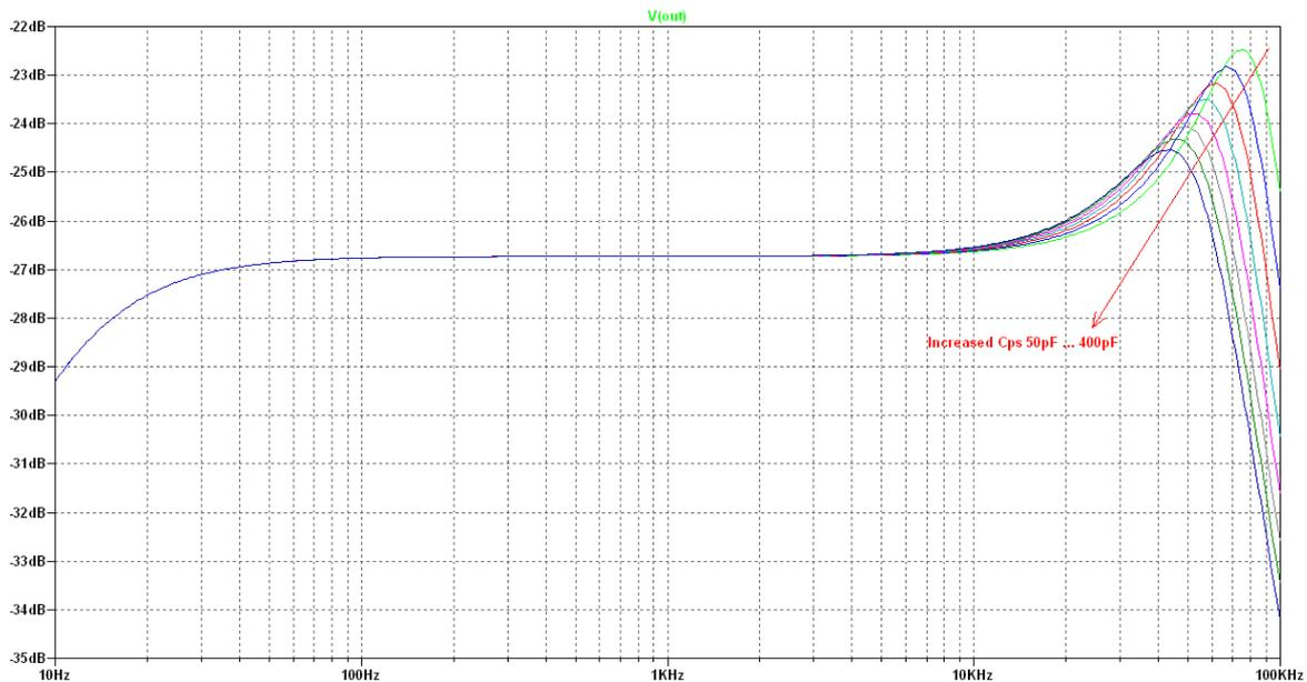
Fig. 9, 10 and 11 Effect of stray C and L on cartridge-step up frequency response.
