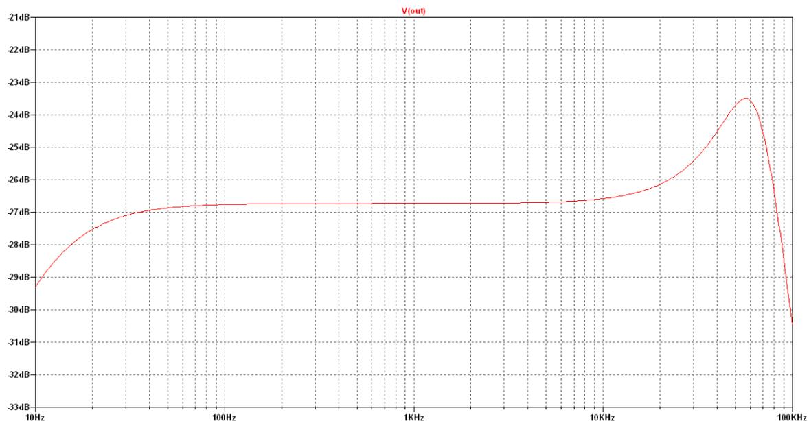
Fig. 2 A resonance of the cartridge-step up appears at 55kHz.
