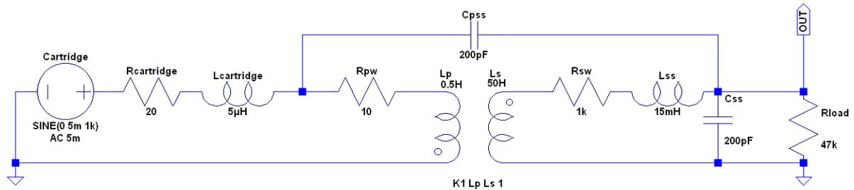
Fig. 1 Cartridge electrical model on the left, transformer model in the middle and loading resistor Rload on the right. 'K1 L<sub>p</sub> L<sub>s</sub> 1' is the spice command that simulates a perfect magnetic coupling of primary to secondary.
