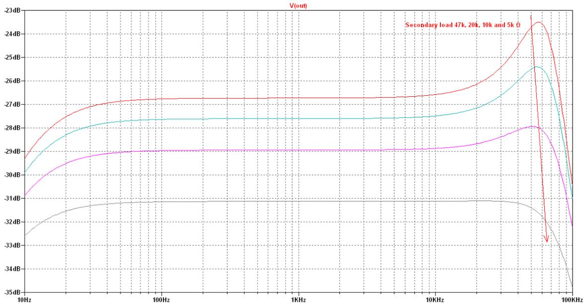
Fig. 5 Effect of reduced load on the cartridge-step up frequency response.
